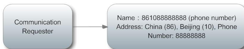
Figure 1 - Addressing Mode NAS (Telecom network)
